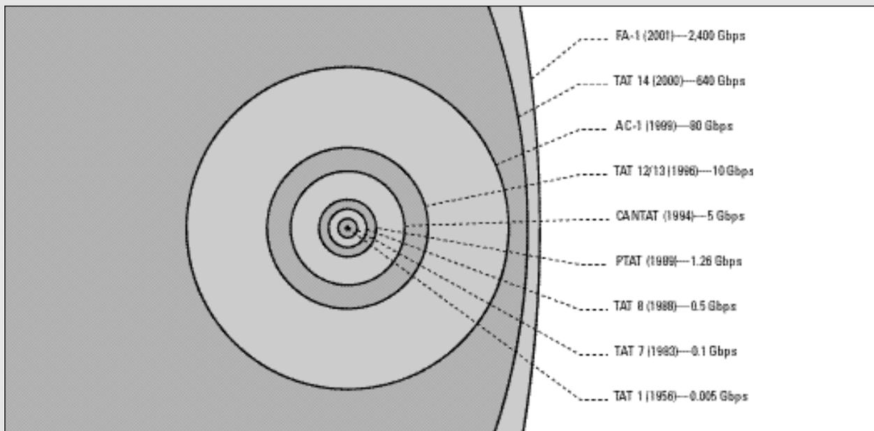
Note: Submarine cables are scaled to capacity when cable was put into service.
